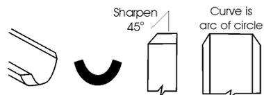
**Spindle Roughing gouge.** An essential tool for between-centre work (spindle turning). This tool quickly reduces square timber to the round. Also ideal for long, shallow curves. Usually 25mm wide.
