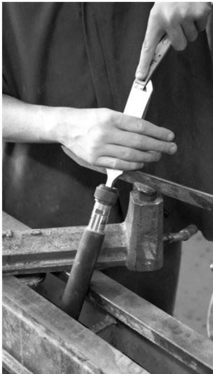
With the hollow grind off a grinding wheel it should be quite easy to see where, on the bevel, you are honing and the slight adjustments needed to rub the paddle on both the front and back of the bevel at the same time. Honing is completed when the cutting edge has a shinier
