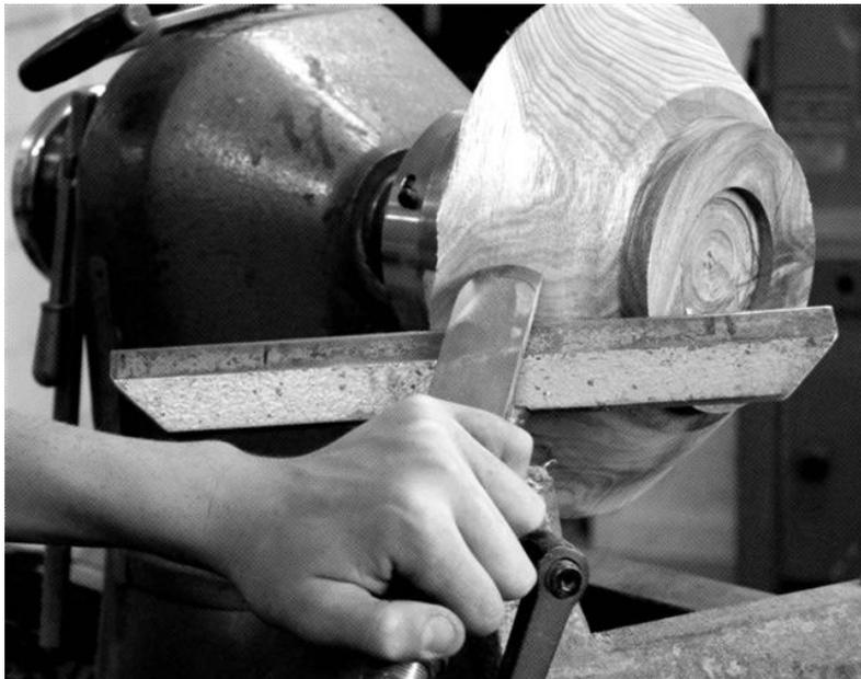
With the lathe going take gentle cuts. If the tool is sharp you should notice fluffy shavings coming off the wood. Best results will be achieved when working with the grain.
