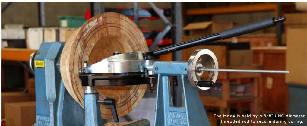
The Max4 is held by a 3/8" UNC diameter threaded rod to secure during coring.
