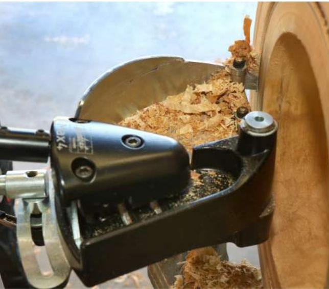
When coring hard and dense wood there is a risk of binding and the lathe stalling. This can be prevented by cutting a wide channel on the inside of the bowl to create more clearance for the cutter. Create the wider channel by backing out of a cut to clear chips, then pull slightly on the cutter when going back to the cut and then retract and push on the cutter bar getting back to the cut. This provides an extra 1/64" clearance on each side.
