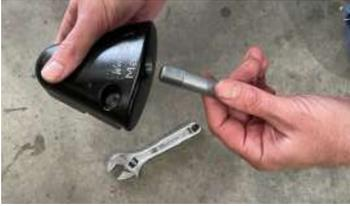
Then screw the Handle Clamp into the Handle, tightening screws with Hex keys in your kit bag.
