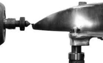
3. Position the Tool Post so the Blade cutter is centered with the point of the drive spur, or slightly above as illustrated (this assumes that when the Blade is extended in the End Grain of the wood that the Blade is now at center). Tighten the Tool Rest locking handle. Slide the shaft collar down the support post and then tighten the grub screw.
